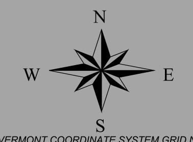
VERMONT COORDINATE SYSTEM GRID NORTH APPROXIMATE MAGNETIC DECLINATION 16 DEGREES WEST
